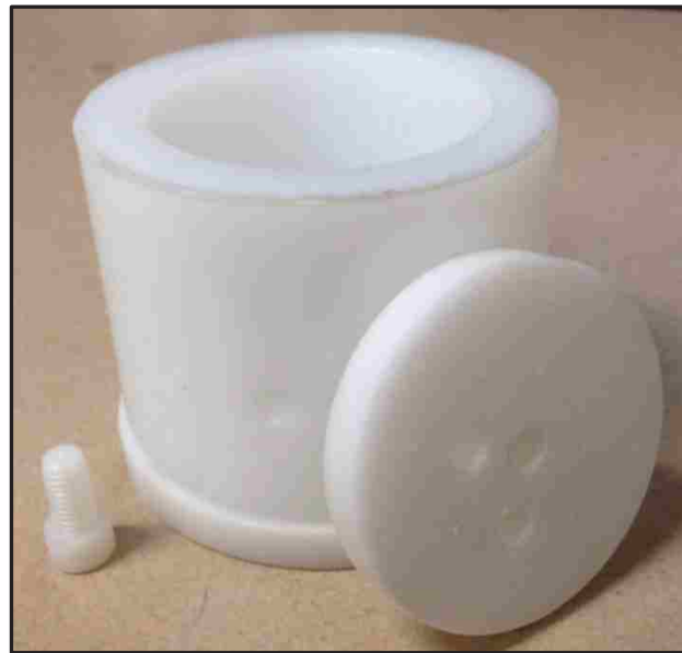
(b) Photo of oedometer cell (top cap and bottom plate, with threaded holes for sensor mounting).
